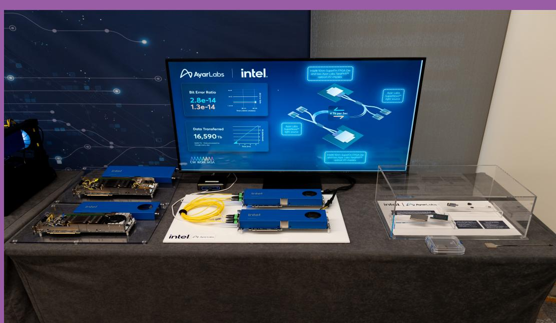
Ayar Labs' optical I/O solution integrated and working in the same package with Intel's Agilex FPGA PCIe card.
